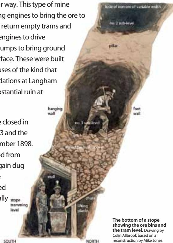
The bottom of a stope showing the ore bins and the tram level. Drawing by Colin Allbrook based on a reconstruction by Mike Jones.
